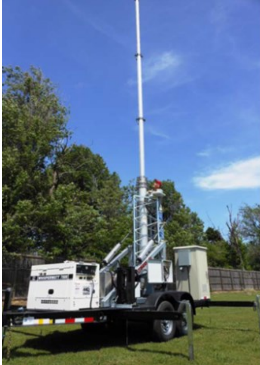
Figure 3.13. Transportable tower & GS.
