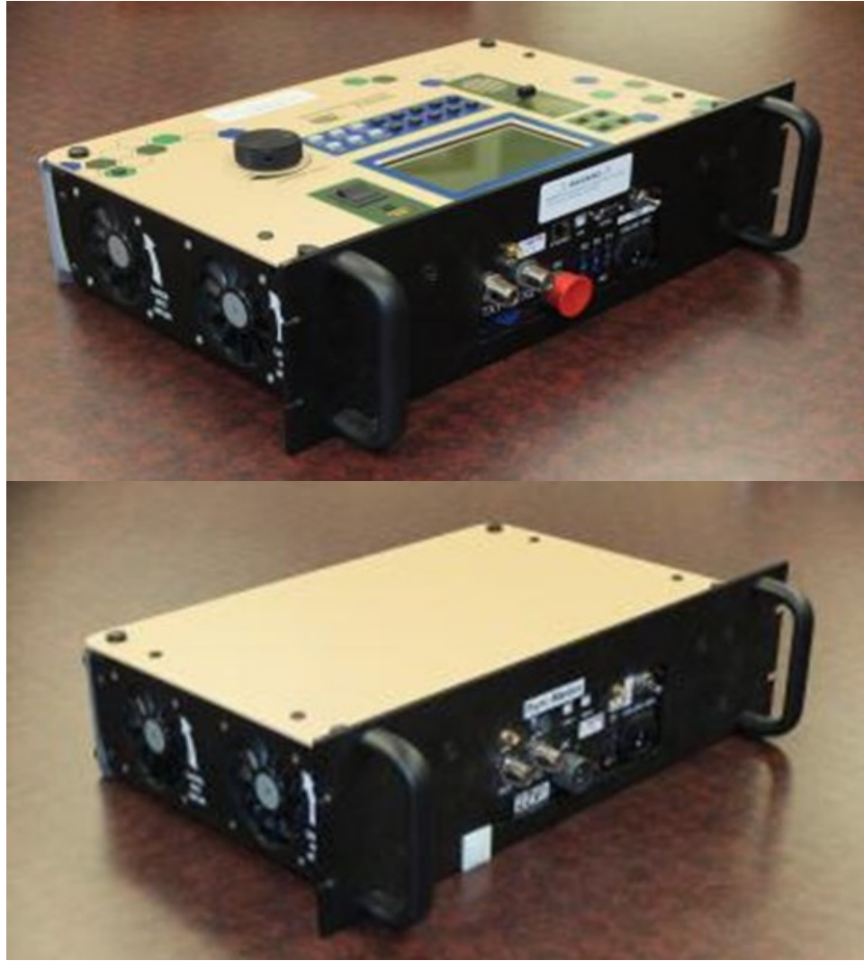
Figure 3.10. Sounder Tx (left) and Rx (right, 1 of 2).
