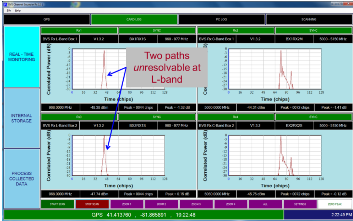
Figure 3.30. “Screen shot” of sounder IR in back-to-back testing; left: L-band, right: C-band [8].
